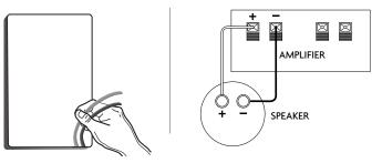
Place the speaker into the hole and press tightly against drywall with one hand, and tighten each of the screws until the speaker is firmly in place. Before placing grille on speaker, make sure there are no vibrations when playing. If so, check the installation screws to see if they need further tightening.
