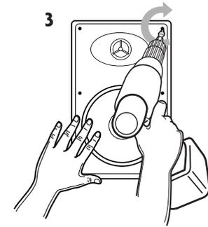
Before placing grille on speaker, make sure there are no vibrations when playing. If so, check the installation screws to see if they need further tightening
