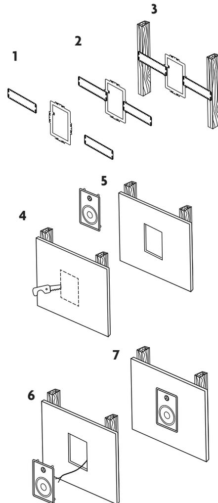
For existing walls, make sure the speaker cutout is placed between two joists with plenty of clearance. Use a stud finder to locate joists, and mark locations. Be sure to avoid electrical wires and plumbing when cutting hole for installation. If you encounter electrical wiring or plumbing, you may have to consider another location (See illustration below).
